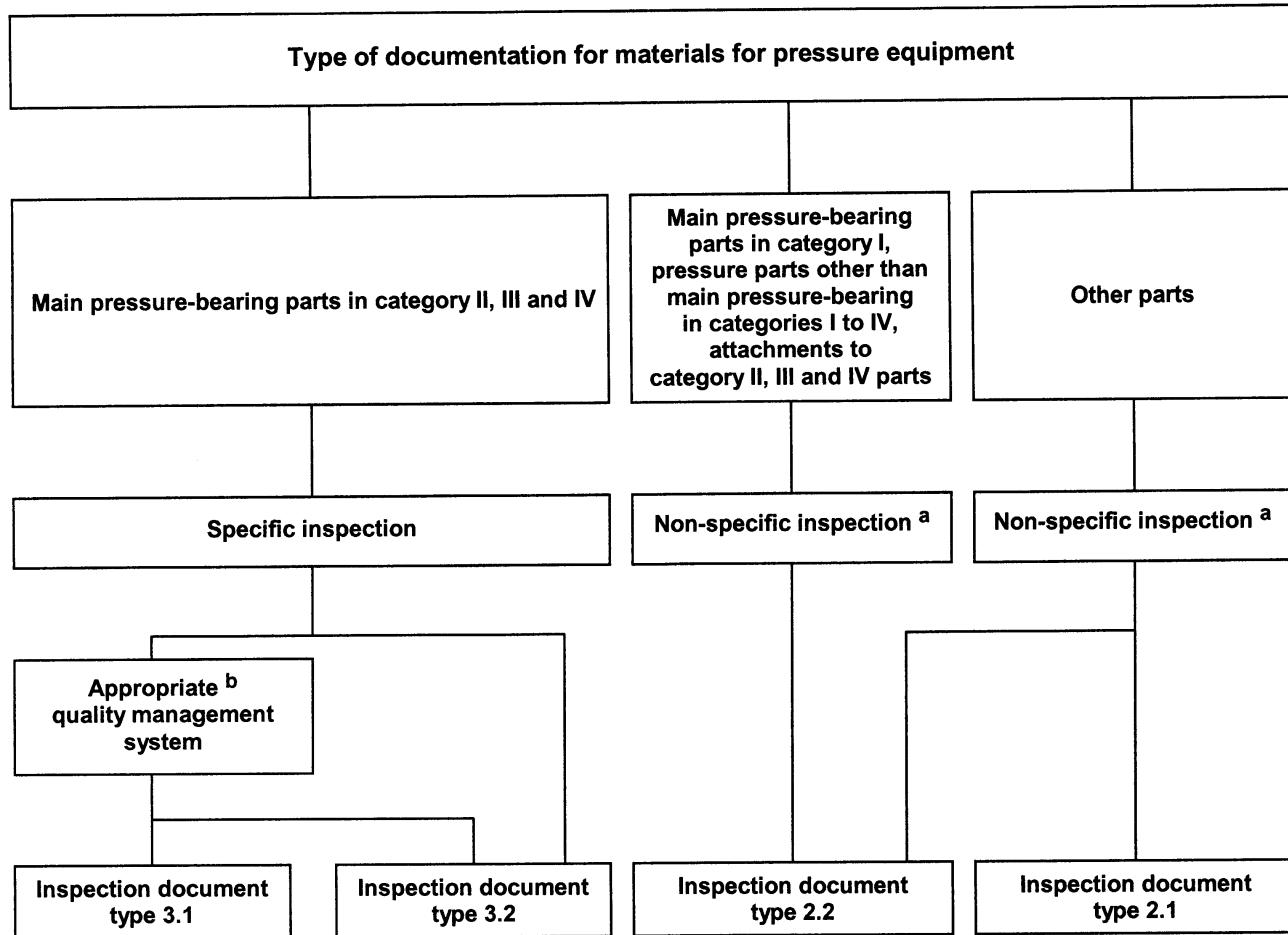
a Non-specific inspection may be replaced by specific inspection if specified in the material standard or the order.
