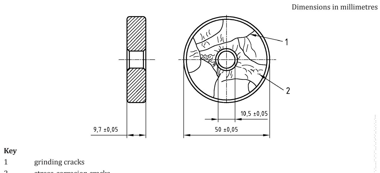
**Figure B.1 — Typical reference block type 1**
