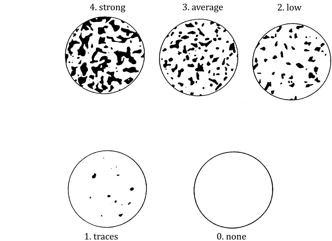
**Figure C.1 — Evaluation of corrosion marks**
