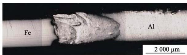
图2 2A11铝合金与201不锈钢焊接接头宏观形貌 Fig.2 Cross-sectional micro-graph of 5A05 aluminum alloy and 201 stainless steel
