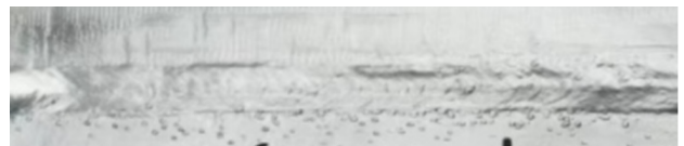
图 13 280 N 压力下的接头表面宏观形貌 Fig.13 Macro-morphology of joint surface under 280 N pressure
