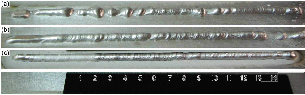
图 2 不同预热次数下单层单道沉积形貌 (a)未预热,20℃;(b)预热一次,50℃;(c)预热两次,100℃ Fig. 2 Morphologies of single layer deposited under different preheating times (a)no preheat,20℃;(b)preheat once,50℃;(c)preheat twice,100℃
