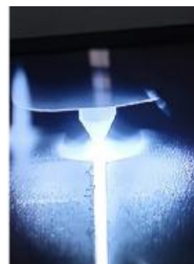
图 2 K-TIG 焊电弧形态 Fig.2 The arc shape of K-TIG welding
