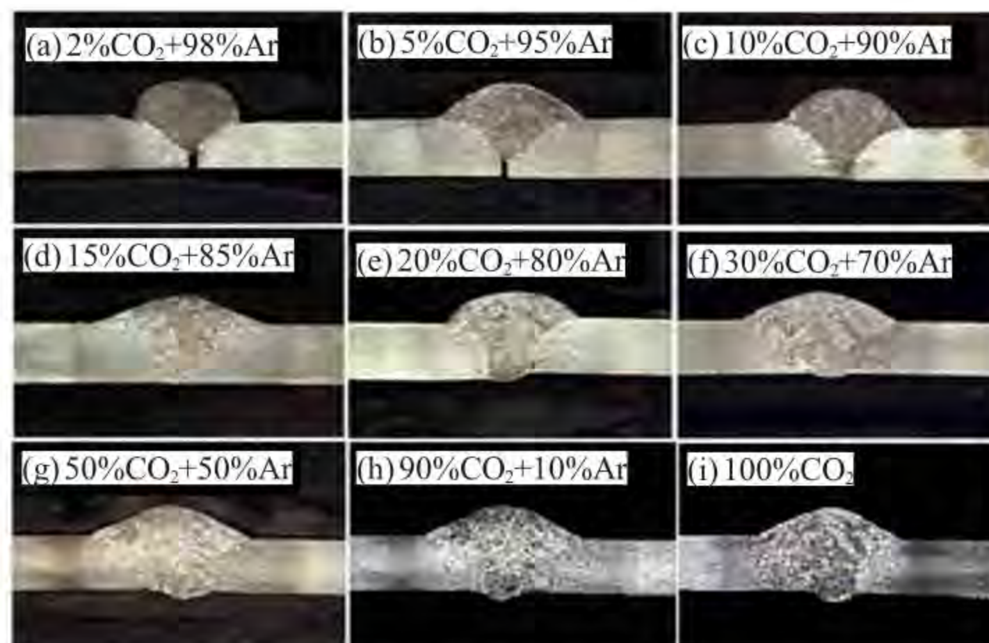
图5 不同保护气体成分下的焊缝截面形貌 Fig.5 Cross-sectional morphologies of the weld beads under different contents of shielding gas
