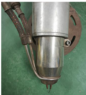
图 3 Tandem 双丝焊枪图 Fig.3 Diagram of Tandem dual wire torch
