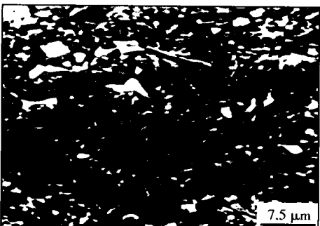
(b) Morphology of lath martensite and retained austenite
