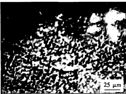
图 1 TIG 焊焊缝金属腐蚀后表面形貌 Fig.1 Micro-appearance of TIG weld surface after corrosion
