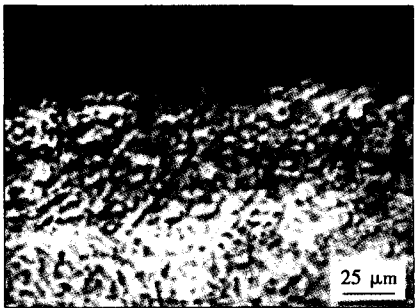
图 2 A-TIG 焊焊缝金属腐蚀后表面形貌 Fig.2 Micro-appearance of A-TIG weld surface after corrosion
