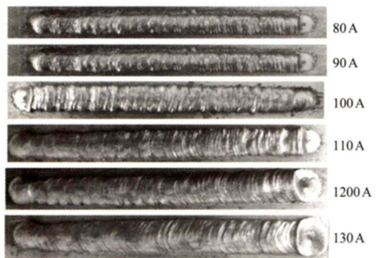
图5 不同电流下焊缝成形 Fig.5 Weld forming under different currents
