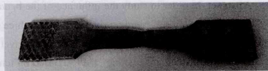
图9 拉伸试样缩颈 Fig.9 Shrinkage of tensile specimen
