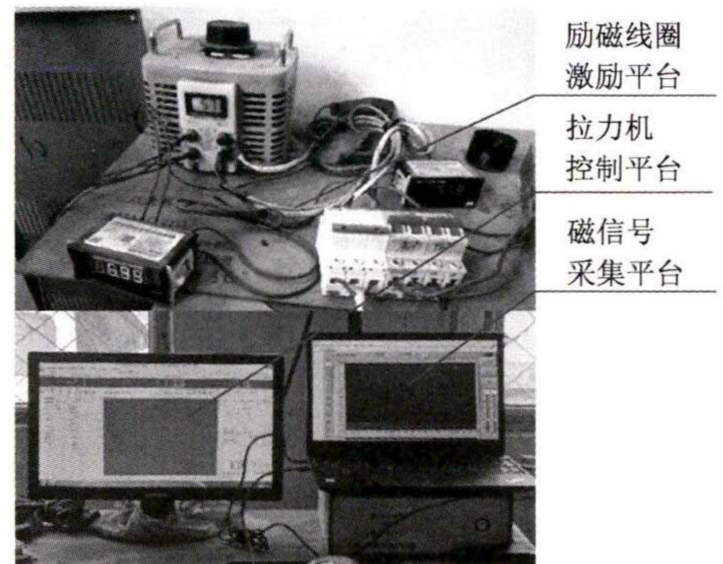
(b) 拉力机控制平台与磁信号采集平台 (b) Tension machine control platform and magnetic signal acquisition platform
