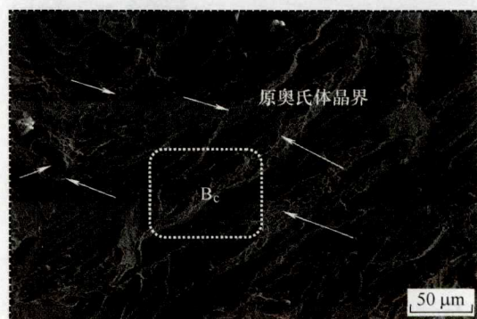
(a) 柱状晶焊缝断口形貌
