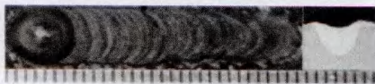
图8 激光功率 2 200 W 时激光熔覆层形貌和剖面 Fig. 8 Morphology and cross-section shapes of single cladding with laser power 2 200 W in single laser heat source cladding
