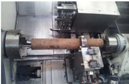
图3 坡口加工实物图 Fig.3 Physical view of groove machining
