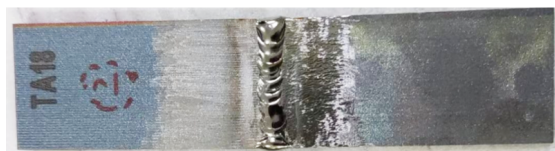
图 4 焊接接头宏观形貌 Fig.4 Macromorphology of weld joint
