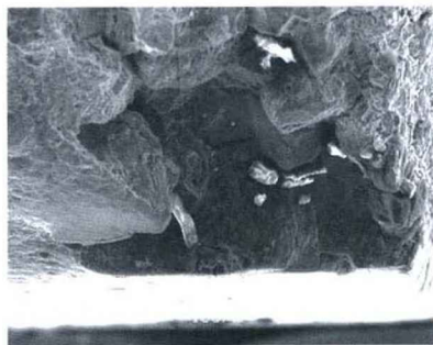
图8 2号试样裂纹断口原始裂纹区沿晶断裂特征 Fig.8 Intergranular fracture characteristics of 2nd sample original crack area
