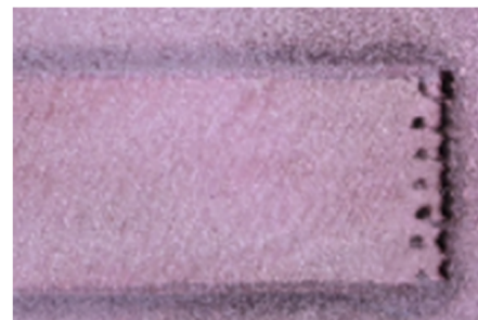
图7 堆焊焊缝区气孔检测结果 Fig.7 Test result of porosity in the weld seam area of the surfacing welding
