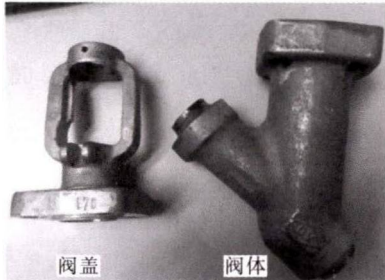
图 1 泄漏阀门的阀体和阀盖 Fig.1 Valve body and bonnet of the leaked valve
