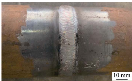
图2 母材热处理后接头表面形貌 Fig.2 Surface morphology of the joint after base material heat treatment
