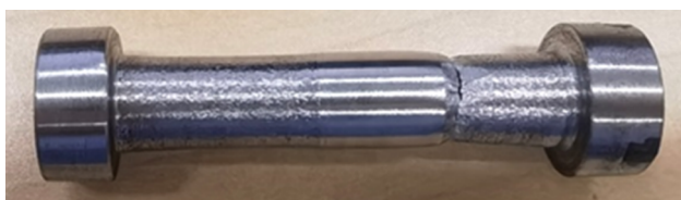
图6 添加中间层的扩散焊拉伸试件 Fig.6 Tensile test piece diffusion welded with intermediate layer
