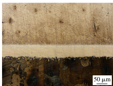
图7 添加中间层的扩散焊缝金相图 Fig.7 Metallography image of diffusion weld with intermediate layer
