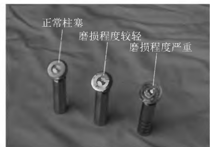
图 10 滑靴磨损柱塞与正常柱塞对比 Fig. 10 The comparison of loose shoe between wear and normal
