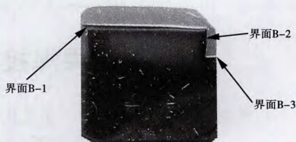
图 4 B 向试样爆炸焊接截面图 Fig.4 Section of explosive welding of B direction
