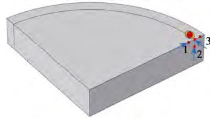
图7 轧辊埋弧堆焊温度采集轨迹 Fig.7 Temperature acquisition track of roll submerged arc welding
