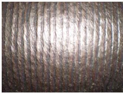
图3 轧辊堆焊焊道形貌 Fig.3 Roll hardfacing weld bead morphology
