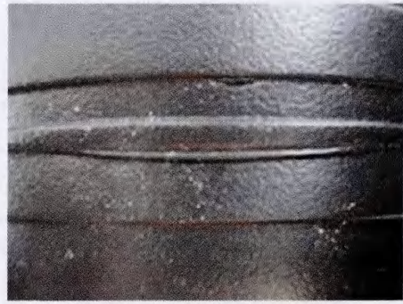
(a) outer surface of failed EF joint
