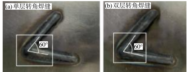
图8 采用转角焊缝模型控制形成的焊缝 Fig.8 Weld forming by using the fillet weld model
