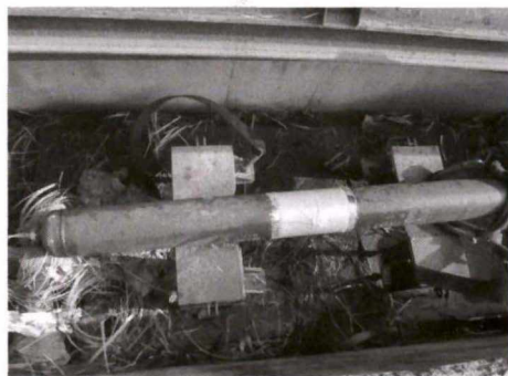
图2 水压试验管件 Fig.2 Test specimen subjected to inner pressure
