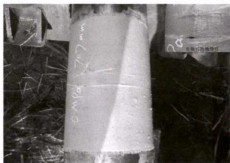
图3 涨破后的缠绕层 Fig.3 Composite layer after burst of the repaired pipe
