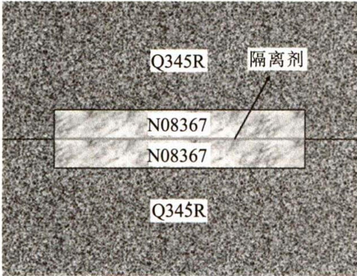
图 1 不锈钢 / 钢复合板的组坯示意图 Fig.1 Schematic diagram of billet formation of the stainless steel/steel clad plates
