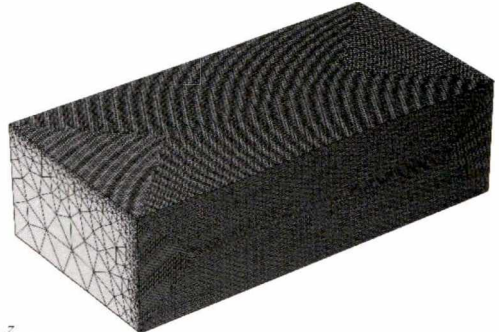
图 4 埋弧堆焊熔池流动几何模型网格划分 Fig. 4 Grid division of flow geometry model of submerged arc surfacing weld pool
