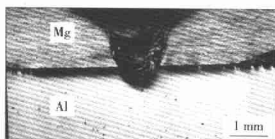
图6 激光-TIG复合热源缝焊镁和铝焊缝横断面形貌 Fig.6 Cross section of laser-TIG hybrid weld bead of Mg and Al
